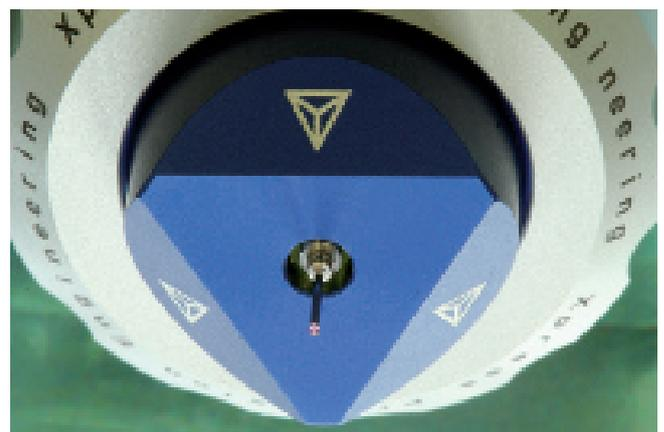
Figure 7. The Gannen XM, the second tactile sensor system produced by Xpress, was designed for 3D measurements of micro-products such as MEMS.
